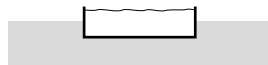
Semi-inground (Attention, the built-in part of the pool requires a lean concrete backfill.)
