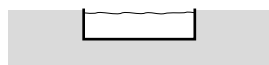
Completely inground (Possible only with a lean concrete backfill (20 – 30 cm.) The pool must always be filled with water, never leave without water for a longer period.
